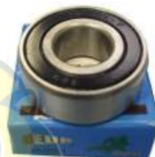
10-202-4 = WAI 10-2021-4 NIPONDENSO LADO COLECTOR CHRYSLER INTER. 15MM, EXT. 35MM X 13MM DE ANCHO
